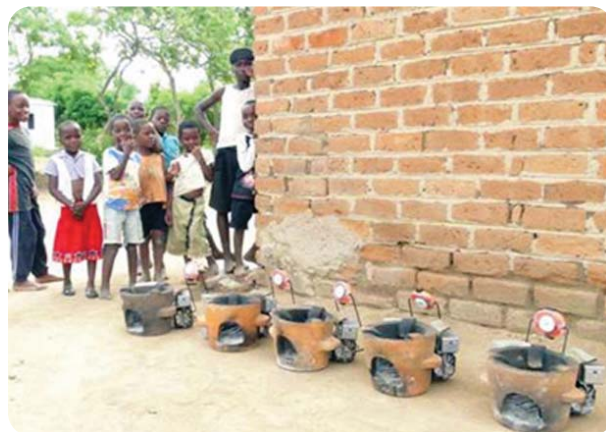
Children from a local village in Malawi admire a new generator designed by energy researchers at the School of Engineering at Trinity College Dublin. The generator generates electricity from cooking stoves, providing lighting and phone charging.
